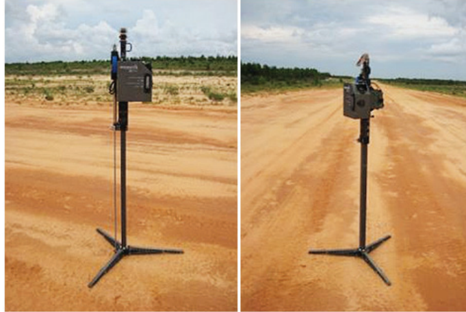
Man-portable automated dynamic cone penetrometer known as the “Mosquito”
